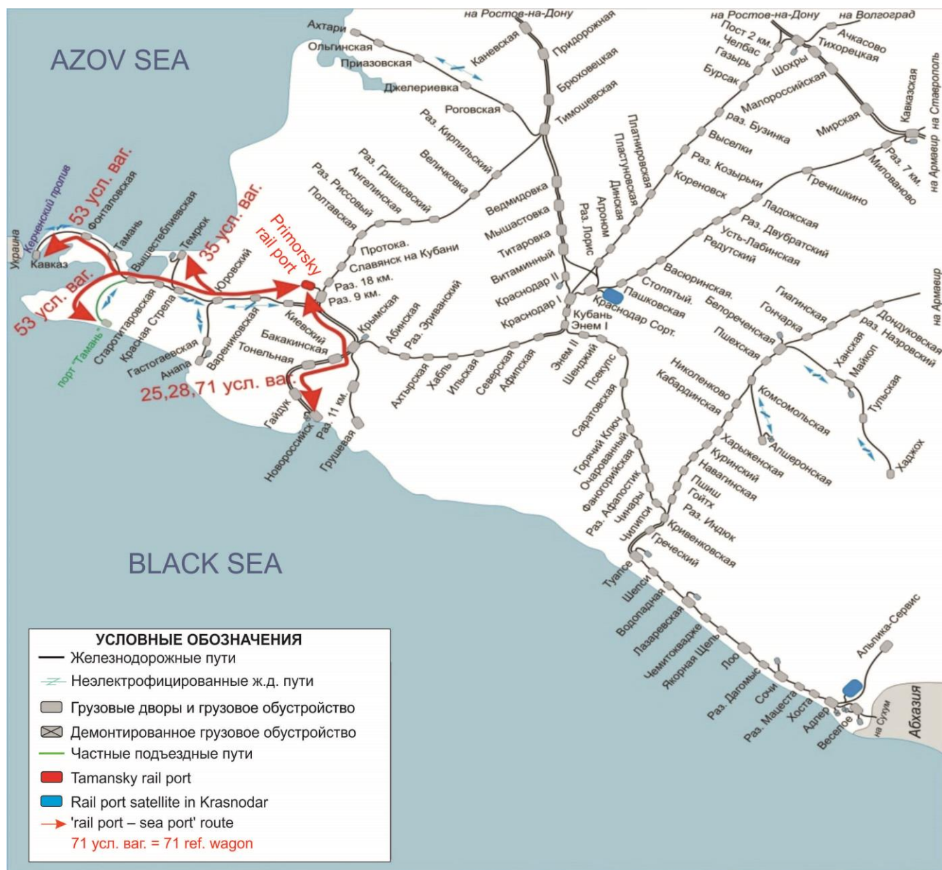
Fig. 5.5. Network of regular block / shuttle trains routes of ‘Tamansky’ rail port connecting relevant seaports of the Azov-Black Sea basin.
